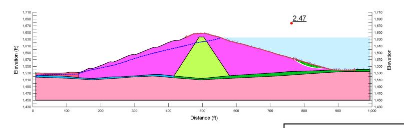
Cross-Section A-A Steady-State Seepage Stability Analysis of Upstream Slope Normal Pool Elevation
