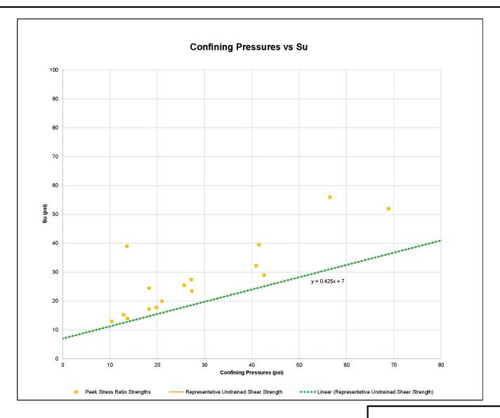
Representative undrained shear strength, c = 1000 psf and  $\phi = 23$  deg.
