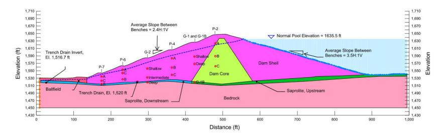
Trench drain is located at elevation 1520 ft.; however, the trench drain is modeled with a total water head set at 1535 ft. to account for the efficiency of the trench drain.
